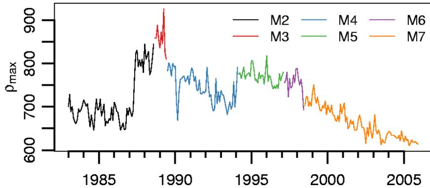
**Figure 4.** Temporal evolution of the 95th percentile ( $\rho_{max}$ ) of the observed reflections for MVIRI, covering 1983 to 2005. The different MVIRI instruments (M 2-7) are coloured for a better distinction. Image from Posselt et al. 2011
