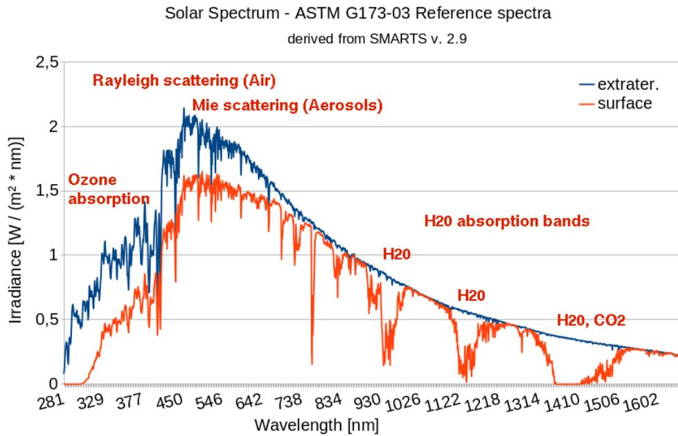
**Figure 2.** Illustration of the solar ~~irradiance~~ irradiance spectrum at the top of atmosphere (extraterrestrial irradiance) and the surface for cloud free skies. The main processes leading to the attenuation of irradiance are shown in the associated spectral range.
