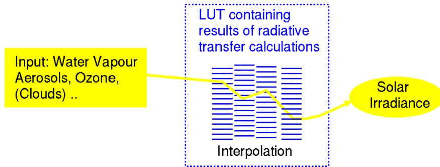
**Figure 1.** The principle of an LUT approach. The transmission is pre-calculated for a variety of atmospheric states with a radiative transfer model (RTM) and saved in a look-up table (LUT). The LUT is then used to determine SSI based on the input given for the atmospheric state for each pixel and time step by interpolation.
