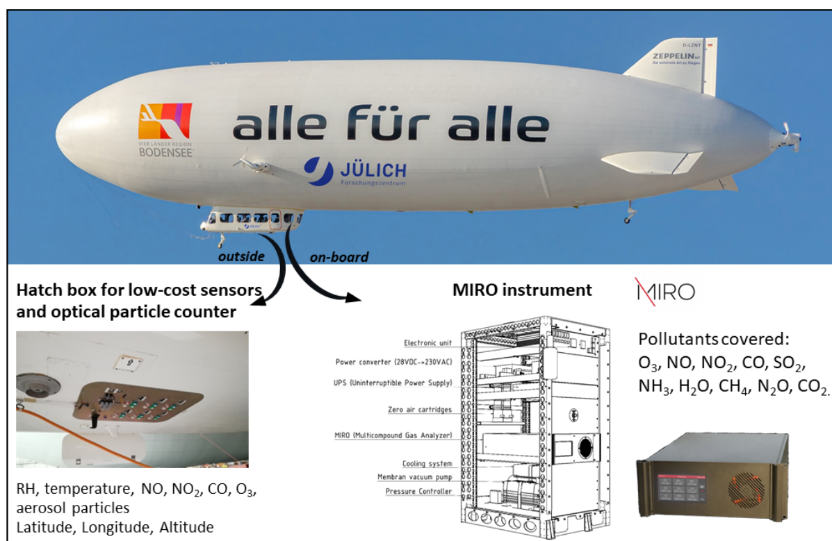
170 Figure 2: Instrumentation onboard the Zeppelin aircraft. (Zeppelin picture by Michael Häfner)
