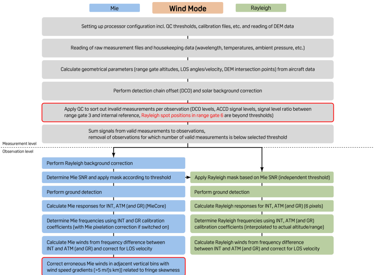
Figure 4. Flow chart of the A2D wind retrieval. Refinements that were introduced in the course of the AVATARE and AVATARI data analysis are indicated as red-framed boxes. INT: internal path; ATM: atmospheric path; GR: ground return.
