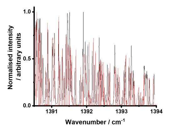
Normalised observed spectrum (black) for SO<sub>2</sub> with the corresponding normalised spectrum reported on the HITRAN database (red).
