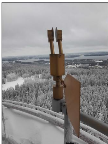
105 Figure 1: ICEMET sensor located in Puijo tower. The height of the ICEMET sensor is 53 cm and the weight is 8 kg. The wind wing is used to align the sensor according to the wind direction (Photo: A. Leskinen).
