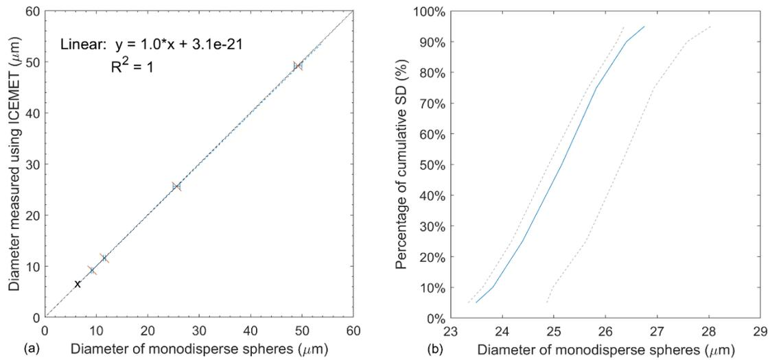
**Figure 3: (a) The results of calibration measurements for ICEMET with a 95% confidence level given by the manufacturer after the size correction was applied as well as 1:1 line (dashed). The 5 μm particles were not certified and therefore the uncertainty value was not defined (black cross). (b) The measured cumulative size distribution using the ICEMET sensor using 25.6 μm monodisperse microspheres. The uncertainty limits specified by the manufacturer are marked as dashed lines.**
