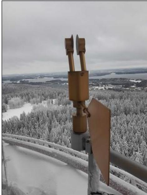
100 **Figure 1: ICEMET sensor located in Puijo tower. The height of the ICEMET sensor is 53 cm and the weight is 8 kg. The wind wing is used to align the sensor according to the wind direction (Photo: A. Leskinen).**
