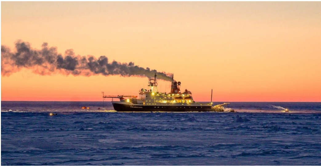
780 Figure A5: A situation when the wind was coming from the stack's direction and the exhaust plume went directly over the Swiss Container , but due to the surface inversion no pollution spikes were measured in the Swiss Container . The container was located at the bow of the ship, below the crane (left hand side in this picture). Photo credit: Ivo Beck.
