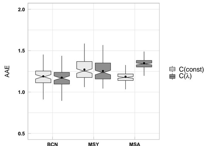
**Figure 7.** The absorption Ångström exponent (AAE) calculated with a constant  $C(\text{const})$  and the wavelength-dependent  $C(\lambda)$  for all stations. Box plots have been obtained as in Figs. 3 and 4, with the markers indicating the mean AAE values.
