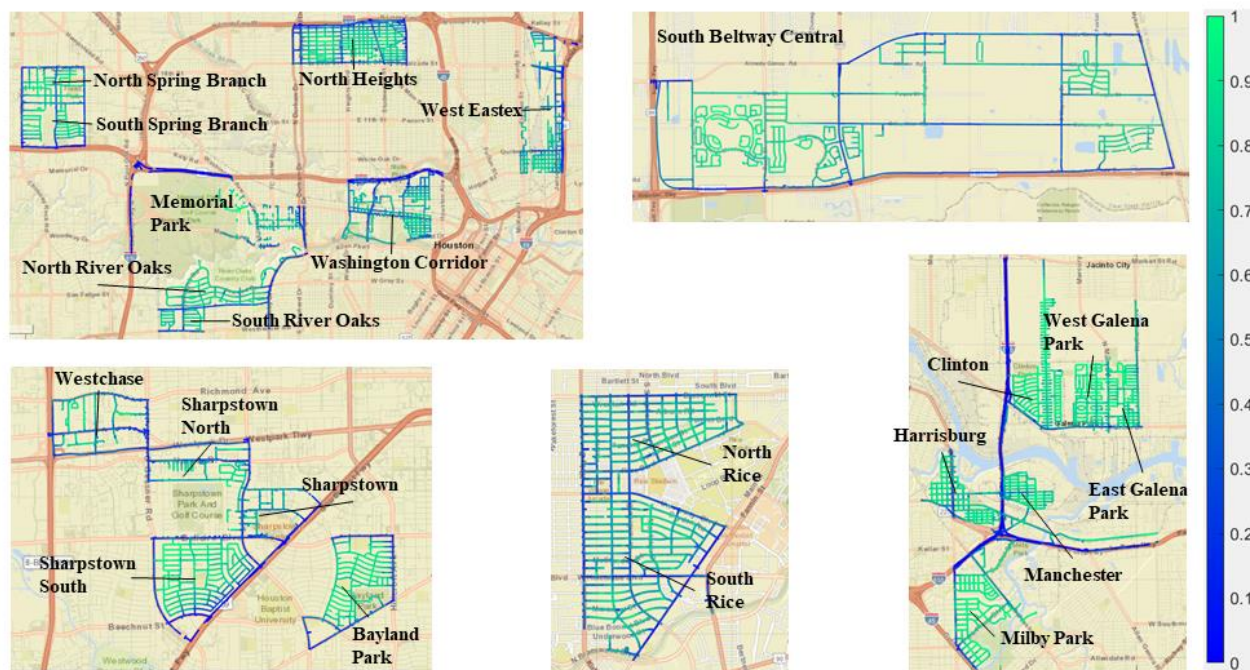
Figure 5. Fraction of points aggregated to road segment network designated as background in SIBaR decoded states for \text{NO}_x . Maps were generated following the methods outlined in Section 2.4. Points are mapped on a scale of 0 to 1; 1 implies all points aggregated to that road segment were designated as background, 0 implies all points were designated as non-background. Details of the census tracts are provided in Table S1. Basemap generated by Matlab geobasemap ‘streets’ and is hosted by ESRI (Sources: Esri, DeLorme, HERE, USGS, Intermap, iPC, NRCAN, Esri Japan, METI, Esri China (Hong Kong), Esri (Thailand), MapmyIndia, Tomtom).
