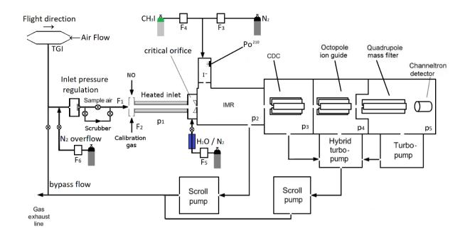
Figure 1 Schematic diagram illustrating the central components of the I-CIMS used in this work. IMR = ion-molecule reactor, CDC = collisional dissociation chamber, F<sub>1</sub> = 1250 cm<sup>3</sup> (STP) min<sup>-1</sup>, F<sub>2</sub> = 50 cm<sup>3</sup> (STP) min<sup>-1</sup>, F<sub>3</sub> = 750 cm<sup>3</sup> (STP)
