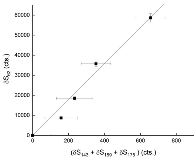
540 **Figure 6:** Relative changes in the sum of signals at  $m/z$  143 ( $\text{IO}^-$ ),  $m/z$  159 ( $\text{IO}_2^-$ ) and  $m/z$  175 ( $\text{IO}_3^-$ ) when adding up to 80 ppbv of  $\text{HNO}_3$ .  $\delta$  refers to the change in signal upon adding  $\text{HNO}_3$  and thus takes background signals at each mass-to-charge ratio into account.
