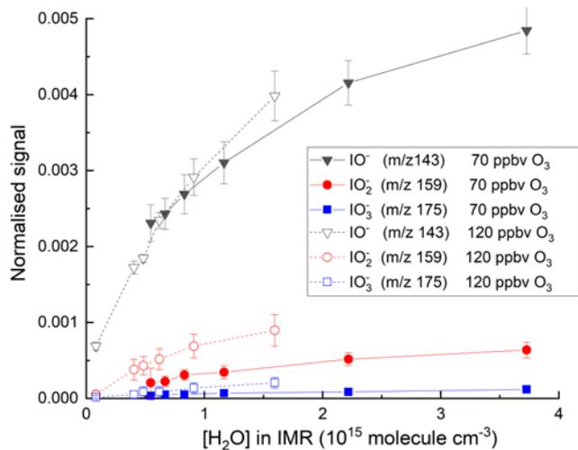
**Figure 4:** Variation in the total ion signal (counts) due to  $\text{IO}^-$ ,  $\text{IO}_2^-$  and  $\text{IO}_3^-$  with the concentration of water vapour in the
