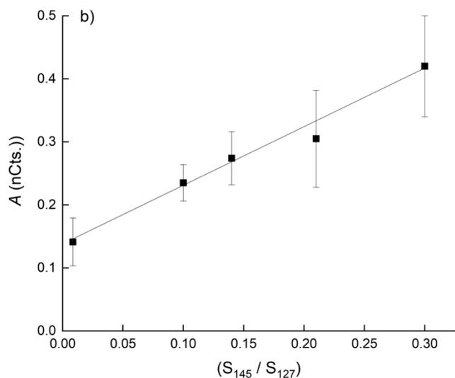
**Figure 7.** a) Dependence of the signal at  $m/z$  62 on the  $O_3$  concentration for 6 different concentrations of  $H_2O$  in the IMR. In the upper 5 curves (solid symbols) the  $HNO_3$  mixing ratio was 38.5 ppbv. In the lowermost curve, the  $HNO_3$  mixing ratio was 18.5 ppbv as indicated. The fits lines are of the form:  $y = A \cdot \exp(1 - \exp(-B \cdot [O_3]))$ . b) Plot of parameter  $A$  versus the relative signal at  $m/z$  145 and  $m/z$  127.
