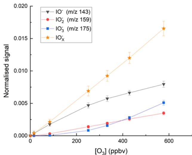
525 **Figure 3:** Variation of the I-CIMS signals at  $m/z$  143 ( $\text{IO}^-$ ), 159 ( $\text{IO}_2^-$ ) and 175 ( $\text{IO}_3^-$ ) with the mixing ratios of  $\text{O}_3$ . The  $\text{O}_3$  mixing ratios are those measured in air before the gas-flow entered the inlet. The water vapour was held constant using our standard setting ( $[\text{H}_2\text{O}]_{\text{IMR}} = 2.9 \times 10^{14} \text{ molecule cm}^{-3}$ ).
