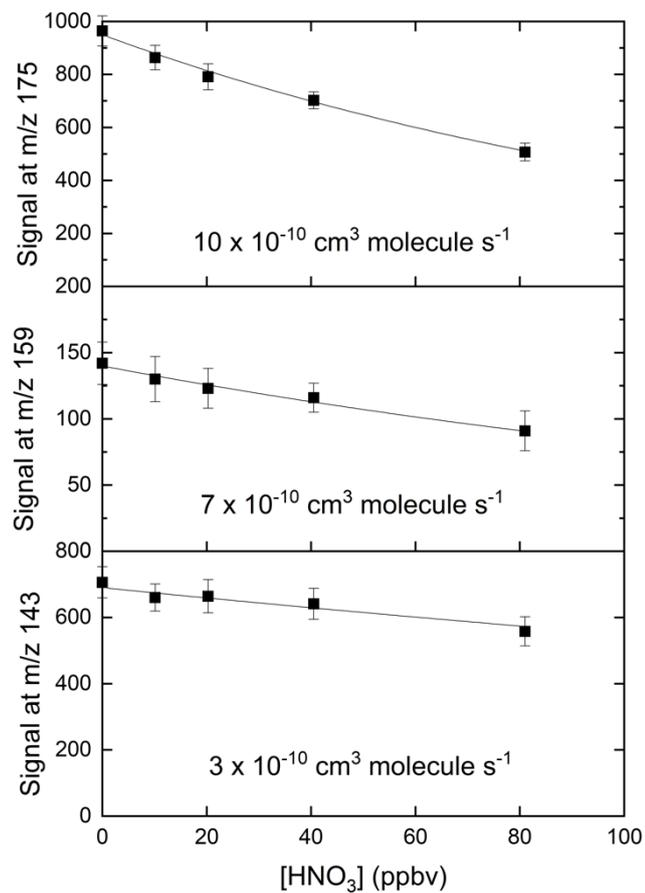
535 **Figure 5:** Relative changes in signals at  $m/z$  143 ( $\text{IO}^-$ ),  $m/z$  159 ( $\text{IO}_2^-$ ) and  $m/z$  175 ( $\text{IO}_3^-$ ) when adding up to 80 ppbv of  $\text{HNO}_3$ . The rate coefficients were calculated using a reaction time of 25 ms and should thus only be regarded as approximate.
