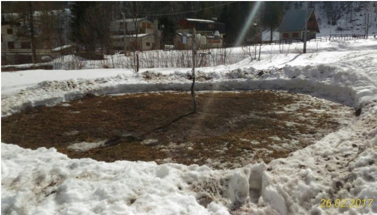
(b) Figure 6Z: (a) The measurement site in its original, un-shovelled snow-covered configuration. In the background position a , where snow will be left. In the foreground position b , with snow still to be removed.
