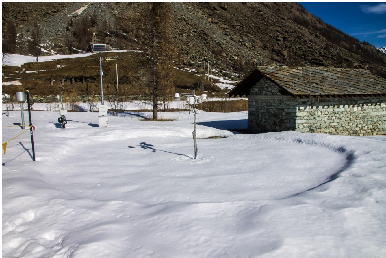
Figure 7: The measurement site in its original, un-shovelled configuration. In the background position a , where snow will be left. In the foreground position b , with snow still to be removed.
