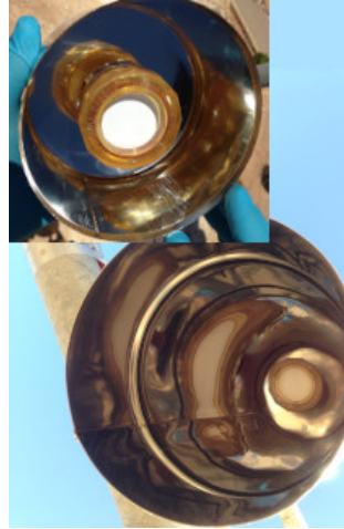
(b) Two bottom-up views of filter on filter holder inside the decanter tube
