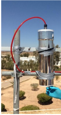
(a) VTD installation on the roof of the building
