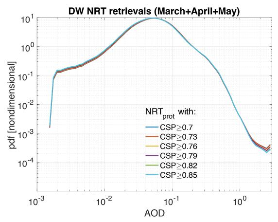
346 Figure 4 Prototype NRT AOD pdfs over dark water surfaces from spring 2020 obtained with different CSP and CSP9 cloud-
