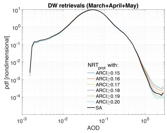
371 Figure 5 Prototype NRT AOD pdfs from spring 2020 obtained with different ARCI thresholds. Data statistic are provided in Table
