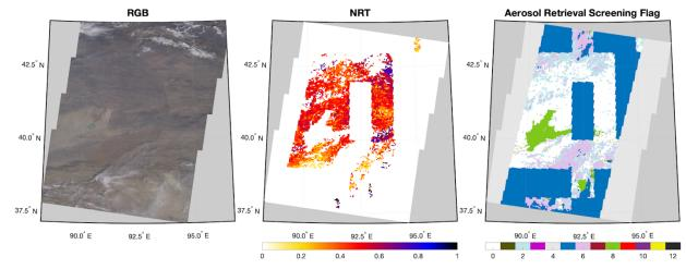
417 Figure 6 Example of snow/ice masking in NRT AOD retrievals. (Left) Visible image of the retrieval area. (Center) Corresponding
