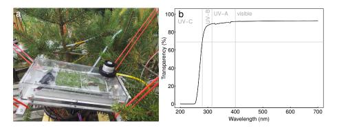
**Figure 2.** Picture of the shoot enclosures used for *PlaSTraGAS* (a) and the UV-VIS transmission spectrum of the transparent chamber cover (b).
