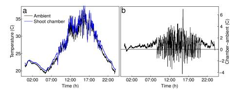
**Figure 4.** Example of the temperature control used with *PlaSTraGAS-gh7*: ambient temperature and temperature in a shoot chamber a the greenhouse compartment (**a**) and the temperature difference between shoot chamber and ambient air (**b**). Data was measured on Aug 1 2019.
