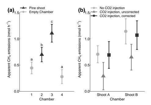
Figure 7. Observed apparent  $CH_4$  fluxes in two empty shoot chambers and two shoot chambers with pine shoots (a). Furthermore, comparison of  $CH_4$  fluxes during chamber closures without and with  $CO_2$  injections (b). Only daytime (illuminated) measurements are included in the figure. Error bars indicate 95% confidence intervals.
