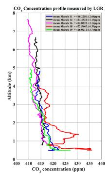
Figure 14: CO<sub>2</sub> concentration profile results measured by greenhouse gas analyzer during aircraft descending flight on different dates. The blue solid line is the result on March 11. The black solid line is the result of March 14. The purple solid line is the result of March 16. The solid red line is the result of March 18. The green solid line is the result of March 19.
