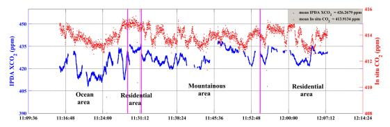
530 Figure 17: XCO<sub>2</sub> comparison results of airborne IPDA lidar and LGR on 14 March 2019. The red scatter is the result of greenhouse gas analyzer. The blue scatter is measured by airborne IPDA lidar. The purplish red vertical line represents the boundary of different surface types. The plane passes through the ocean area, urban residential area, mountain area and urban residential area in turn.
