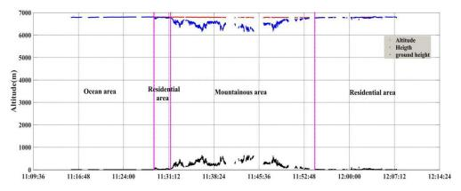
Figure 3: Aircraft flight height and corresponding surface elevation on 14 March 2019. The red dots are the altitude of the aircraft measured by the onboard GPS system. The blue scatter points are the distance measured by lidar. The black scattered points are the difference between the altitude measured by the GPS and the distance measured by the lidar, and also represent the surface elevation. The purple-red vertical line is the dividing line of different surface types.
