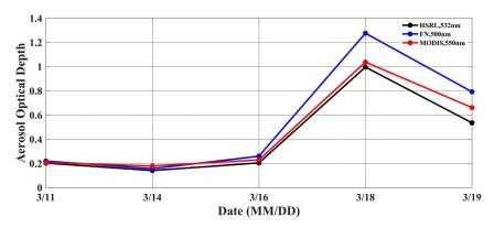
Figure 15: Aerosol optical depth results on different dates. The blue scatter is measured by the sun photometer of Funing ground station. The black scatter is the measurement results of the airborne lidar 532nm channel. The red scattered points are the measurement results of Moderate Resolution Imaging Spectroradiometer (MODIS)
