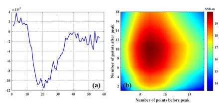
Figure 9: (a) Online wavelength echo pulse signal in ocean area. (b) The change of the SNR of the echo pulse signal in the ocean area with the number of selected pulse points.
