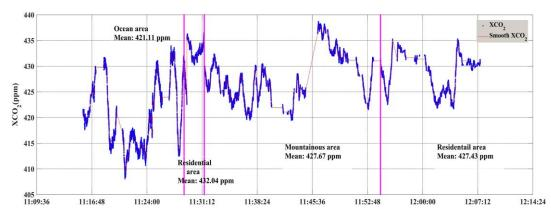
Figure 12: XCO<sub>2</sub> results in ocean, urban residential and mountainous areas on 14 March 2019. The purplish red vertical line represents the boundary of different surface types. The plane passes through the ocean area, urban residential area, mountain area and urban residential area in turn.
