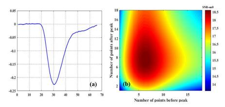
490 Figure 7: (a) Online wavelength monitoring pulse signal. (b) The change of pulse signal SNR with the number of selected pulse points.
