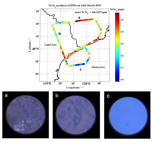
Figure 13: XCO<sub>2</sub> distribution on the flight trajectory and surface photos of typical areas on 14 March 2019. Among them, a represents the urban residential area, b represents the mountain area, and c represents the ocean area.
