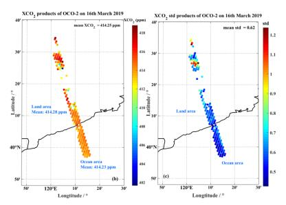
Figure 18: Orbit and detection results of OCO-2 satellite on March 16. The solid red line in figure (a) is the flight path of the aircraft. The yellow mark point is the position of the suborbital point of the OCO-2 trajectory in the flight area (© Google Earth Pro). Figure (b) shows the XCO<sub>2</sub> results detected by OCO-2. Figure (c) shows the corresponding standard deviation.
