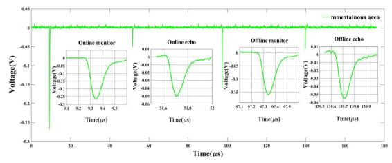
Figure 6: Original echo signal of mountain area (total signal and pulse amplification signal). The amplification signals from left to right are online monitor signal, online echo signal, offline monitor signal and offline echo signal.
