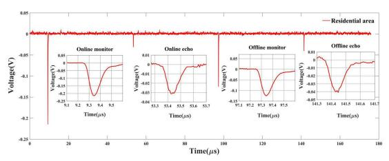
Figure 5: Original echo signal of urban residential area (total signal and pulse amplification signal). The amplification signals from left to right are online monitor signal, online echo signal, offline monitor signal and offline echo signal.
