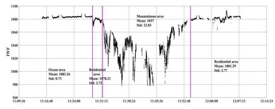
Figure 11: IWF results in ocean, urban residential and mountainous areas on 14 March 2019. The purplish red vertical line represents the boundary of different surface types. The plane passes through the ocean area, urban residential area, mountain area and urban residential area in turn.
