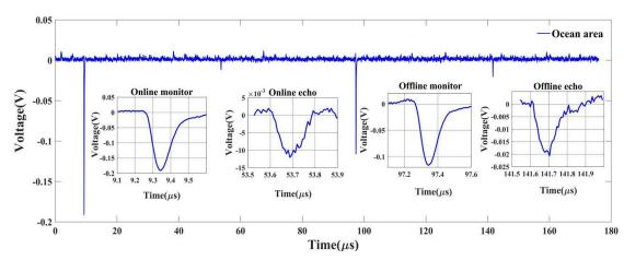
Figure 4: Original echo signal of ocean area (total signal and pulse amplification signal). The amplification signals from left to right are online monitor signal, online echo signal, offline monitor signal and offline echo signal.
