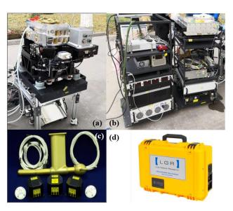
Figure 1: The physical picture of IPDA lidar system. (a) It is the transceiver system, installed in the pod outside the aircraft. (b) It is the control system and data acquisition system of some equipment, which is installed in the sealed cabin of the aircraft. (c) It is the the Aircraft Integrated Meteorological Measurement System (AIMMS). (d) It is a commercial instrument Ultraportable Greenhouse Gas Analyzer, that was installed in an unsealed cabin of the aircraft.
