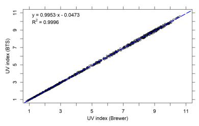
Figure 5: Synchronized UV index obtained from the BTS versus the ones from the Brewer #150. The measurements were derived from cloud-free conditions and SZAs below  $70^{\circ}$  combining all the available data of the three measurement campaigns (711 pairs of UVI values).
