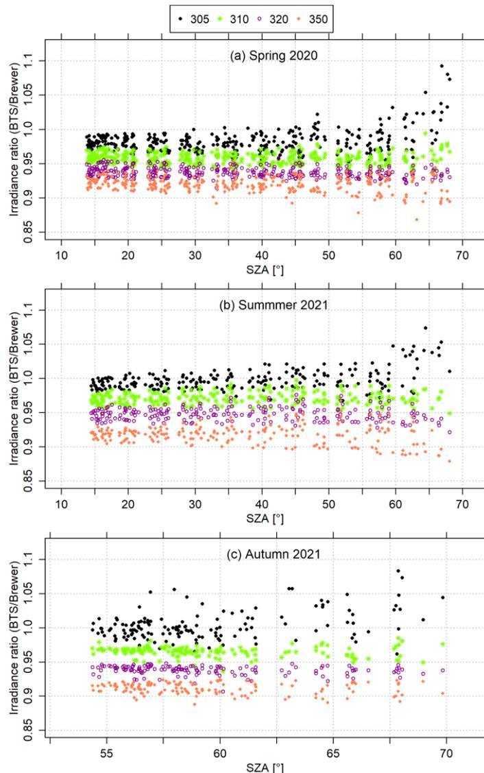
**Figure 3:** The ratios of global UV spectral irradiance at selected wavelengths between the BTS and the Brewer #150. The measurements were obtained from cloud-free conditions and SZAs below 70° during (a) spring 2020, (b) summer 2021 and (c) autumn 2021. Each data point is calculated from the average over a  $\pm 2.5$  nm wavelength band.
