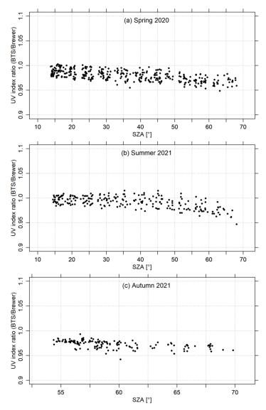
Figure 4: The ratio of UV indices between the BTS and the Brewer #150, as a function of solar zenith angle. The measurements were obtained from cloud-free conditions and SZAs lower than  $70^{\circ}$  during (a) spring 2020, (b) summer 2021 and (c) autumn 2021.
