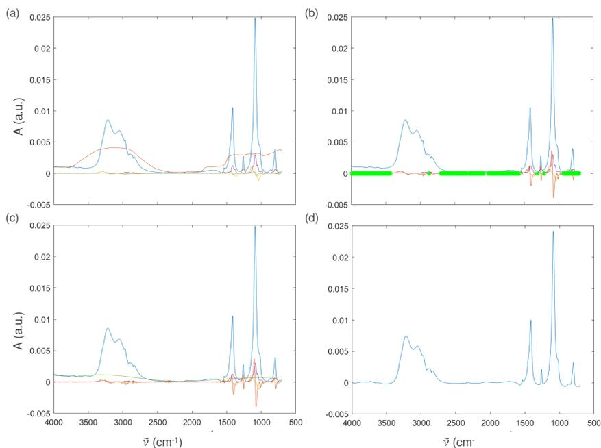
**Figure S4.** (a) Absorbance spectra (blue), moving mean of the absorbance spectra (red), slope of the absorbance spectra (orange), moving mean of the slope (green) and the moving standard deviation of the slope (purple). (b) Identified baseline points (green points). (c) A smoothed spline fitting the baseline points (green), and (d) the baseline corrected spectra.
