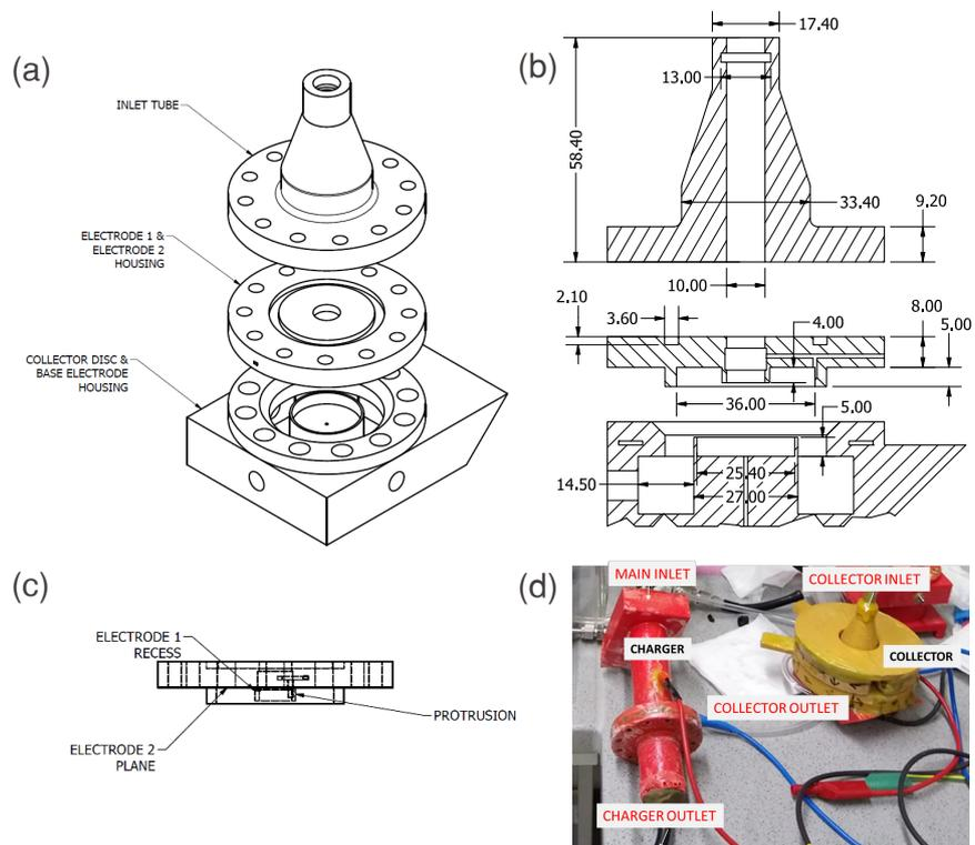
**Figure S2.** (a) Engineering drawing of the device assembly, (b) cross-section view with dimensions (in mm), (c) side view of the electrode housing part with the protrusion visible, and (d) fabricated and assembled device with the different parts labelled.
