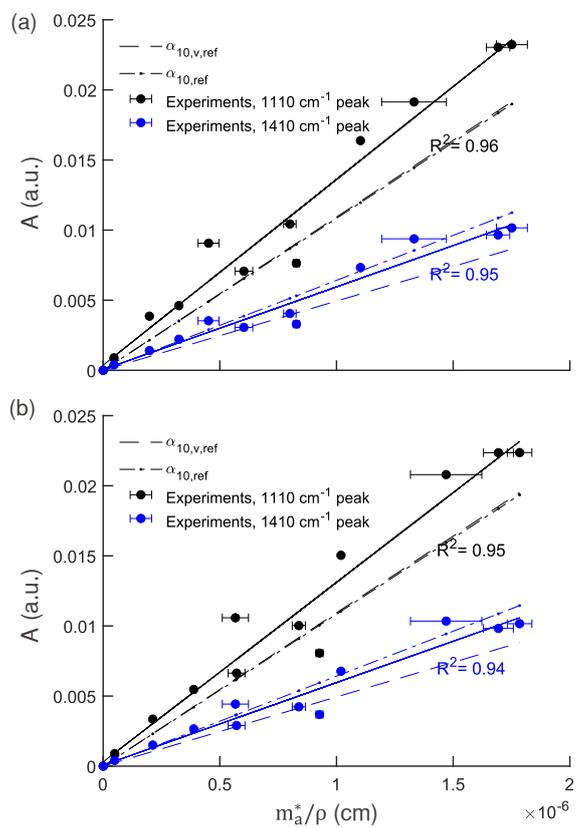
**Figure S6.** (a) Response of IR absorbance ( $A$ ) against the equivalent thickness (cm) calculated assuming  $\phi_R(r_b) = 1$  for absorbance at the peak near 1110  $\text{cm}^{-1}$  (for  $\nu_3(\text{SO}_4^{2-})$ ) and at the peak near 1410  $\text{cm}^{-1}$  (for  $\nu_4(\text{NH}_4^+)$ ). (b) Reproduction of Figure 5b ( $\phi_R(r_b) \neq 1$ ) but using the modified peak heights after removing the PDMS absorption profile (i.e. from the  $\alpha_{10,v}$  calculated in Figure S5b).
