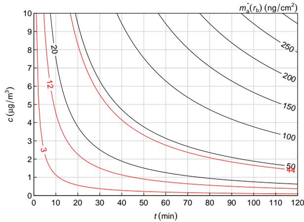
**Figure S9.** Areal mass densities  $m_a^*(r_b)$  in units of  $\text{ng}/\text{cm}^2$  for a given average airborne concentration  $c$  and sampling time  $t$ . Red lines indicate values for 9.5, 20, and 30 dB.
