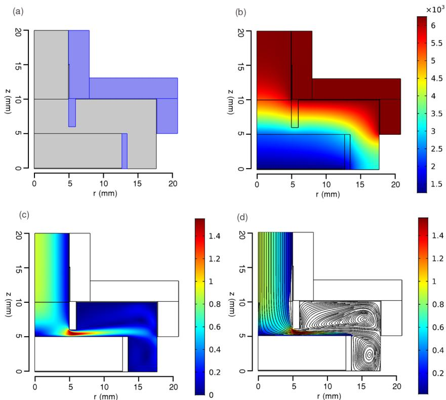
**Figure S1.** Numerical simulations of the ESP device for (a) the device schematic with the outer and inner body (ABS) highlighted, (b) steady state voltage field (V), (c) steady state velocity field (m/s), and (d) particle trajectories in the steady state field at the last time step.
