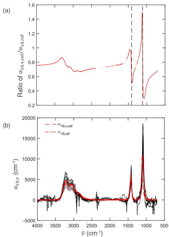
**Figure S5.** (a) Ratio of the reference volume absorption coefficient ( $\alpha_{v,ref}$ ) to the linear absorption coefficient ( $\alpha_{ref}$ ) for ammonium sulfate calculated using  $n$  and  $k$  (Earle et al., 2006). (b) Comparison of modified volume absorption coefficient ( $\alpha_v$ ) adjusted by removing PDMS imaginary refractive index profile (Myers et al., 2001) (scaled by the peak at 800 cm<sup>-1</sup>) from the calculated from the experiments as shown in Figure 5a.
