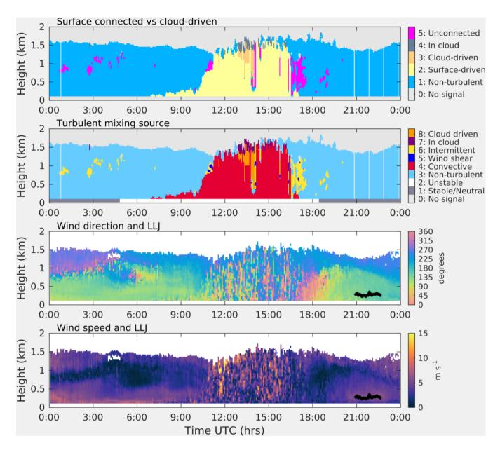
**Figure 4.** Time-height plots of atmospheric boundary layer classification using the Manninen et al. (2018) scheme showing (a) whether mixing is connected to the surface or cloud driven and (b) the turbulent mixing source, together with time-height plots of (c) wind direction and (d) wind speed on 28 August 2017 at Jülich, Germany. The black lines on the two lower panels show low-level jet (LLJ) altitude (Tuononen et al., 2017).
