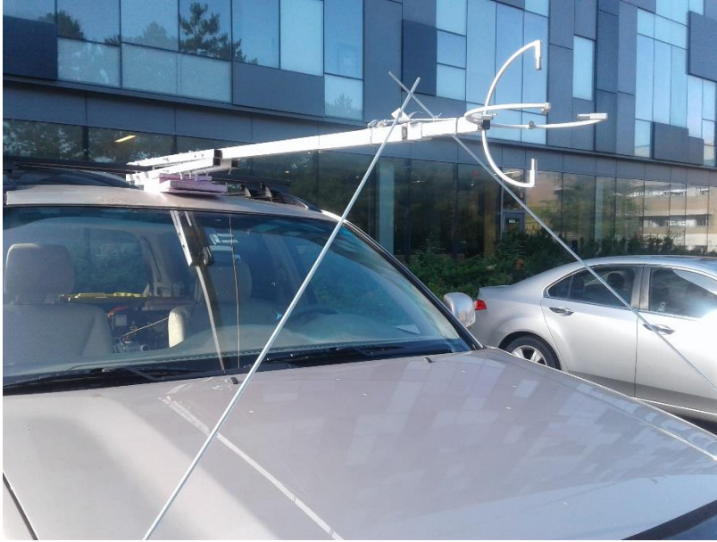
70 Figure 1: A front view of instrumented car (also referred to as a mobile car platform or mobile car laboratory) used in this investigation.
