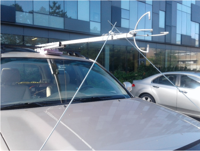
Figure 1. A front view of instrumented car (also referred to as a mobile car platform or mobile car laboratory) used in this investigation.
