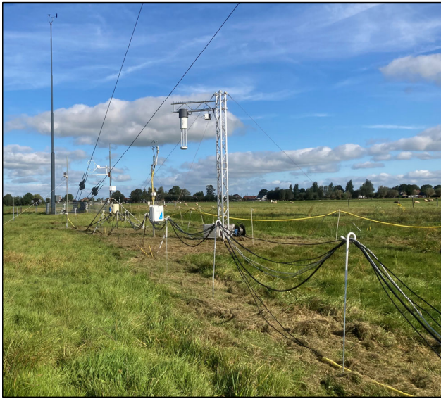
210 Figure 2. The instruments, seen from the miniDOAS container looking north. From left to right: 10 m wind vane mast, mast with the two retroreflectors of the miniDOAS instruments, mast with sonic #3, mast with sonic #1 and LI-7500DS; mast with HT8700E and its cooling unit. Sonic#2 was placed later at 40 cm on the southeast side of HT8700E on the same mast (not shown in the photo). The 213 m mast is off to the right (east).
