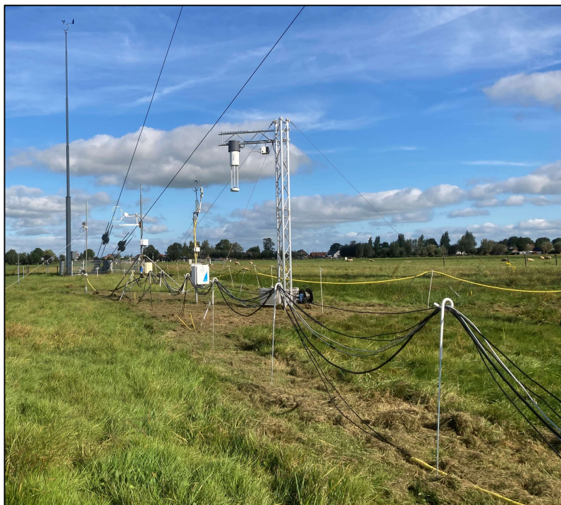
165 Figure 2. The instruments, seen from the miniDOAS container looking north. From left to right: 10 m wind vane mast, mast with the two retroreflectors of the miniDOAS instruments, mast with sonic #3, mast with sonic #1 and LI-7500DS; mast with HT8700E and its cooling unit. Sonic#2 was placed later at 40 cm on the southeast side of HT8700E on the same mast (not shown in the photo). The 213 m mast is off to the right (east).
