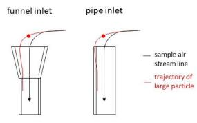
→ Larger particle would impact into pipe wall due to inertia without the funnel
