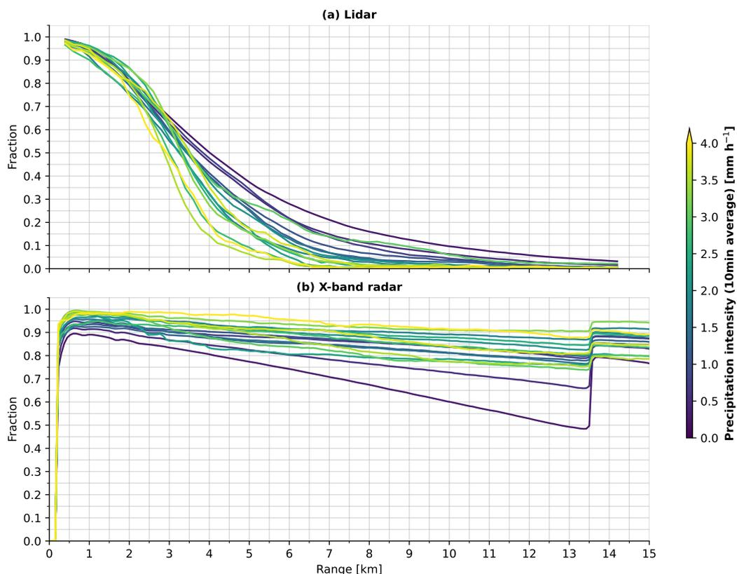
**Figure 12.** Same as Fig. 6, but as a function of precipitation intensity, separated into different precipitation classes. Each line corresponds to a precipitation intensity class with a bin width of  $0.25 \text{ mm h}^{-1}$
