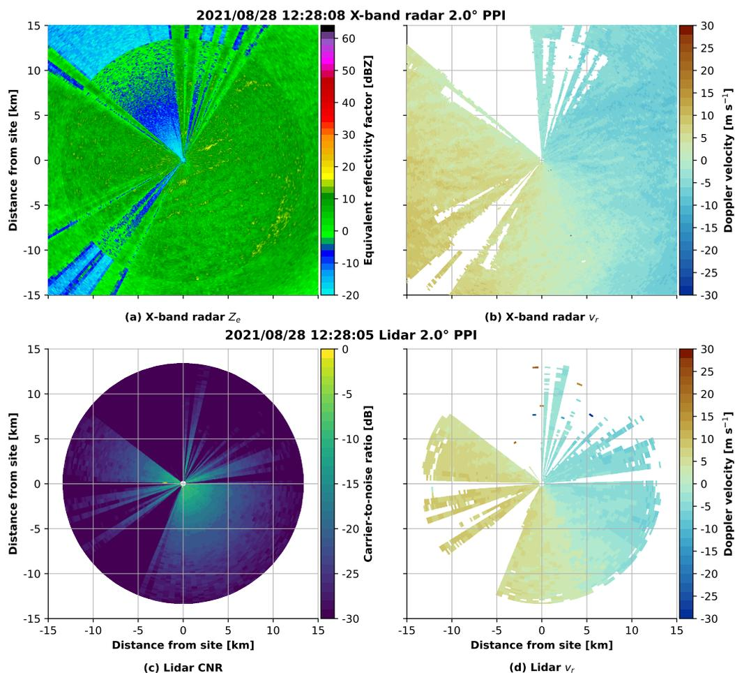
**Figure 7.** Data example from August 28th 2021 at 12:28 UTC showing PPI scans at 2° of X-band (a) radar reflectivity and (b) Doppler velocity, and Doppler lidar (c) carrier-to-noise ratio (CNR) and (d) Doppler velocity. Doppler velocity colour map is from Crameri (2021).
