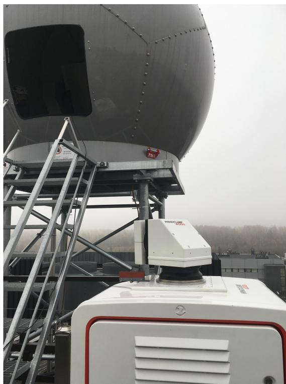
**Figure 1.** Vaisala WRS400 X-band radar and WindCube400S Doppler lidar installed on the roof of a building at Vaisala Oyj headquarters in Vantaa, Finland. Photo taken by Raisa Lehtinen.
