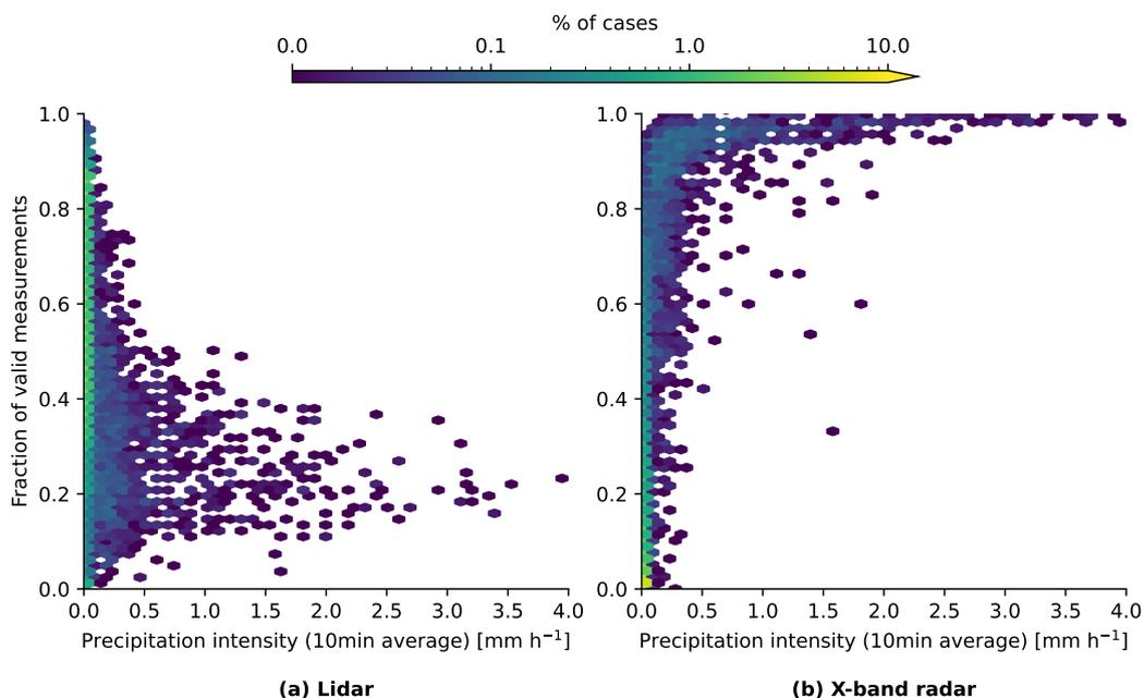
**Figure 11.** Fraction of valid measurements as function of precipitation intensity (10-minute average, optical) for (a) Doppler lidar and (b) X-band radar Doppler velocity measurements.
