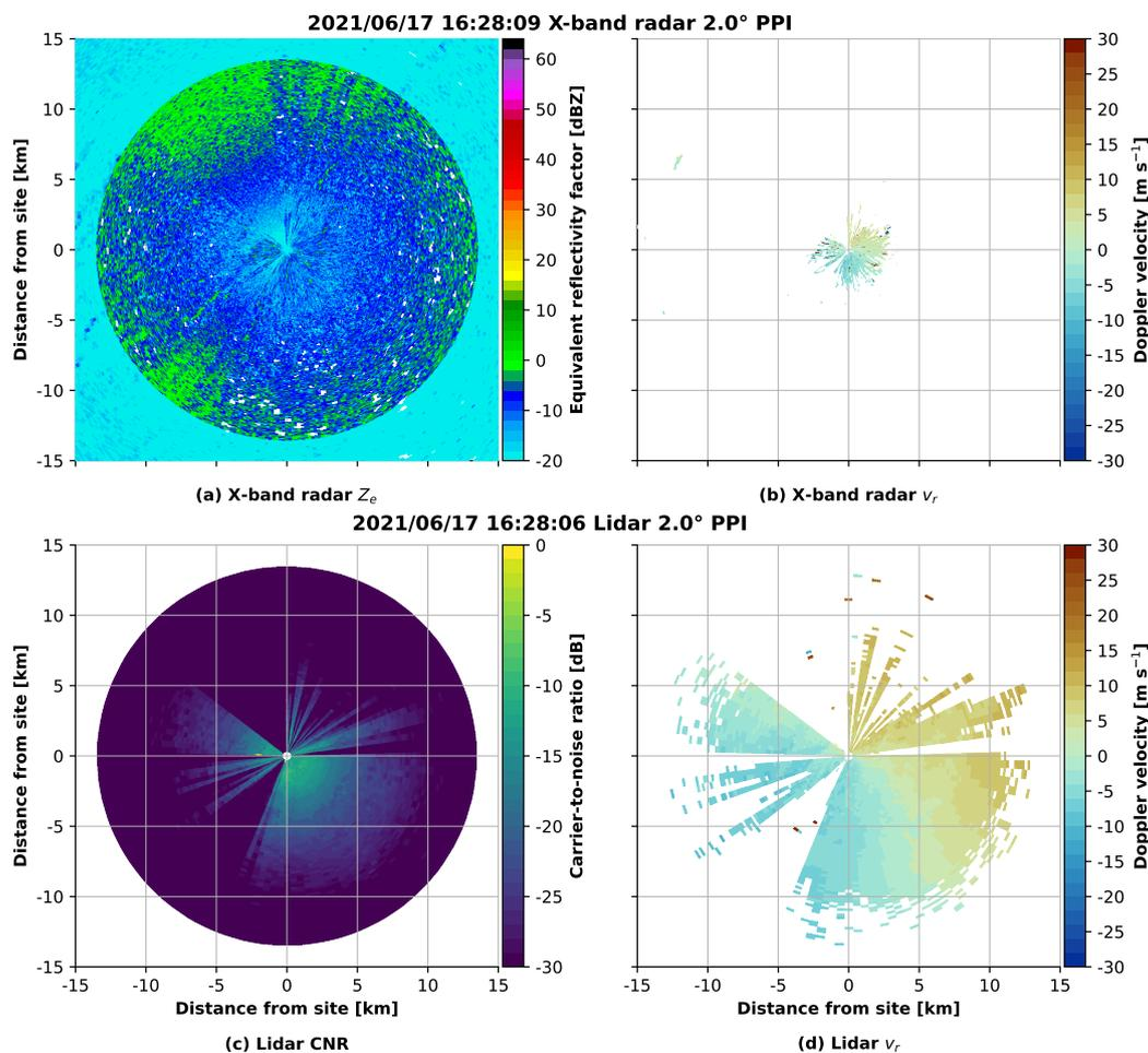
**Figure 8.** Data example from June 17th 2021 at 16:28 UTC showing PPI scans at 2° of X-band (a) radar reflectivity and (b) Doppler velocity, and Doppler lidar (c) carrier-to-noise ratio (CNR) and (d) Doppler velocity. Doppler velocity colour map is from Crameri (2021).
