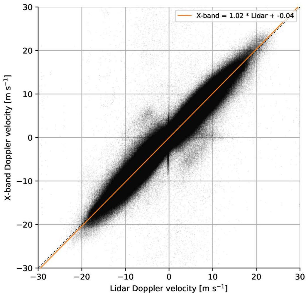
**Figure 3.** Scatterplot of Doppler lidar versus X-band radar radial Doppler velocity measurements. The orange line indicates the linear fit to the data and the black dashed line indicates the one-to-one agreement.
