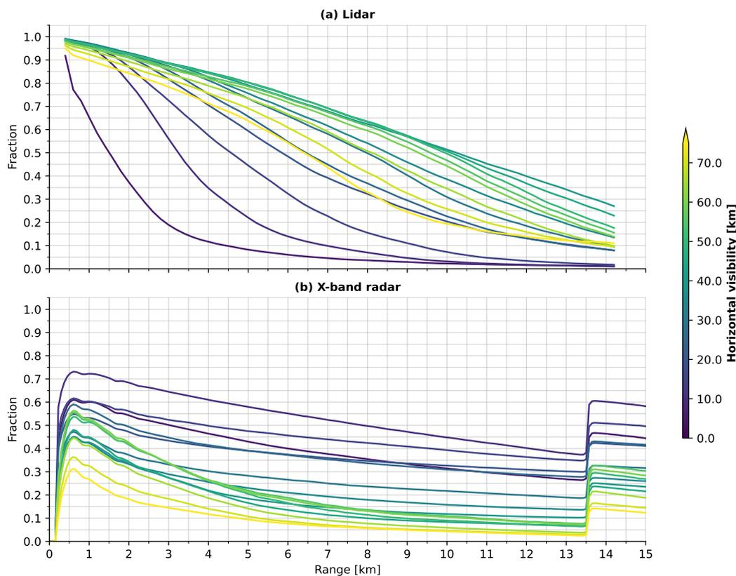
**Figure 6.** Fraction of available measurements as a function of measurement range for (a) Doppler lidar and (b) X-band radar calculated separately for different horizontal visibility classes. Each line corresponds to a horizontal visibility class with a bin width of 5000 m.
