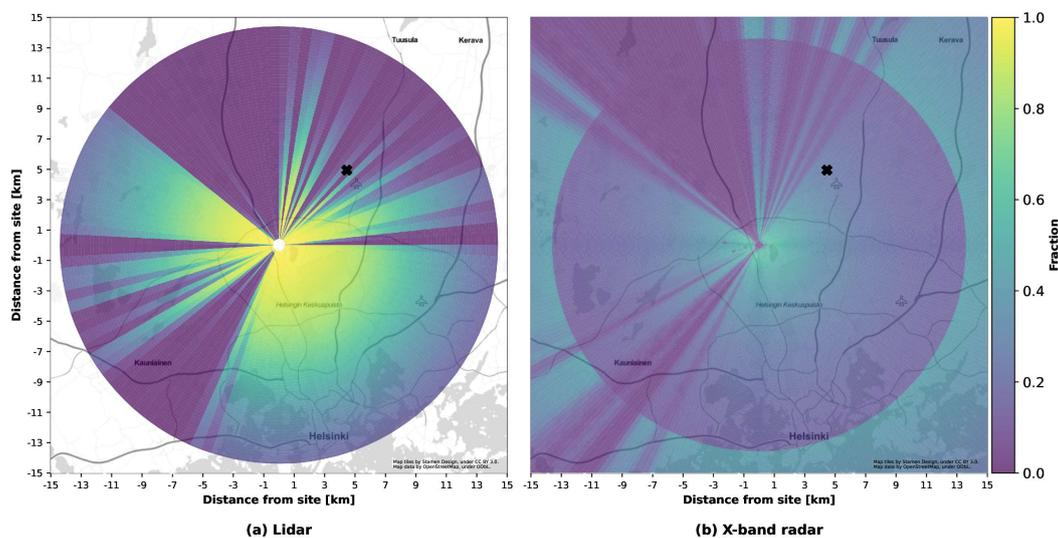
**Figure 2.** Fraction of available measurements during the entire measurement campaign for (a) lidar and (b) X-band radar. The location of the surface weather station is marked with a black cross. Background map tiles by Stamen Design, under CC BY 3.0. Map data by OpenStreetMap, under ODbL.
