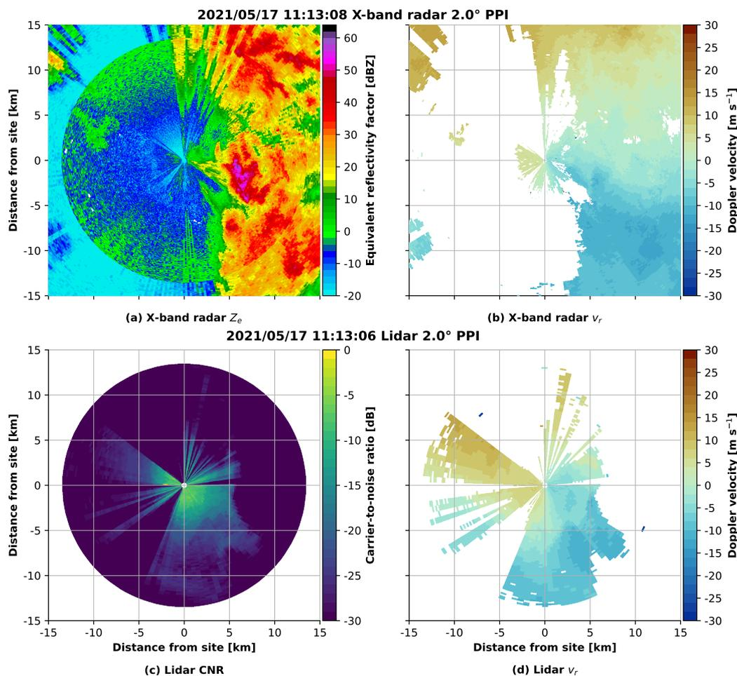
**Figure 13.** Data example from May 17th 2021 at 11:13 UTC showing PPI scans at 2° of X-band (a) radar reflectivity and (b) Doppler velocity, and Doppler lidar (c) carrier-to-noise ratio (CNR) and (d) Doppler velocity. Doppler velocity colour map is from Crameri (2021).
