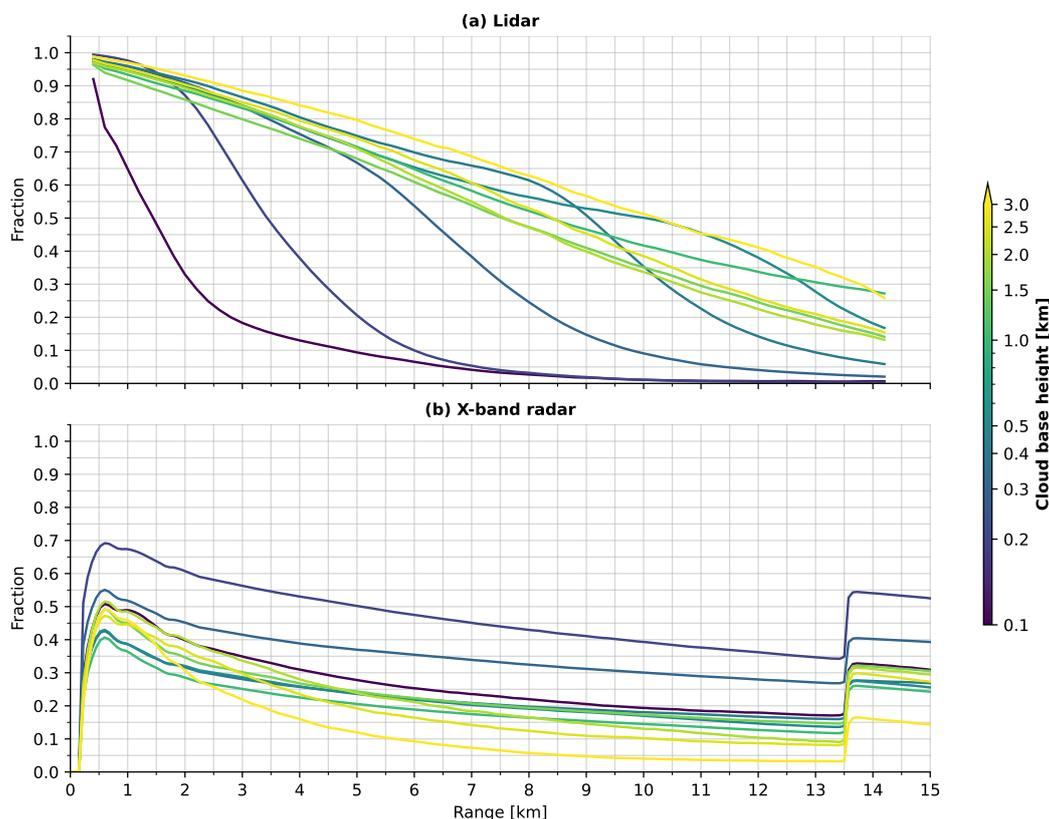
**Figure 10.** Same as Fig. 6, but as a function of cloud base height, separated into different cloud base height classes. Each line corresponds to a cloud base height class with a bin width of 100 m below 500 m and a bin width of 500 m above. The line colour indicates the upper limit of the bin. Note the logarithmic scale for the colour bar.
