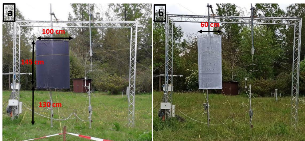
Fig. 1. Two examples of shroud experiment setup containing two upsides down sonic anemometers and two high precision pressure transducers with the quad disk to measure static pressure. (a) A 1 m diameter cylindrical shroud with fine porosity gray color texture (b) A 60 cm cylindrical shroud with a white insect screen.
