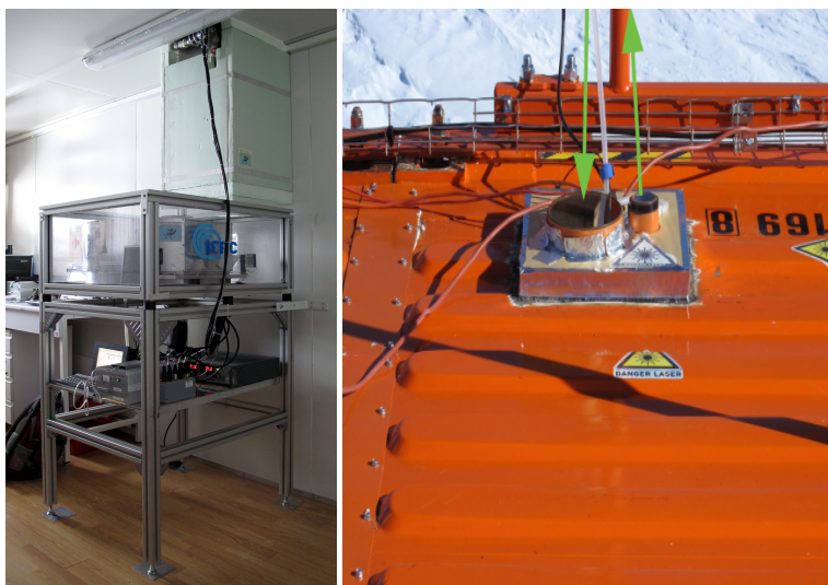
Figure 1. Left side: REFIR-PAD Fourier transform spectroradiometer inside the PHYSICS shelter with the 1.5 m chimney connecting the instrument with outside. Right side: output windows of the tropospheric lidar on the roof of the shelter.
