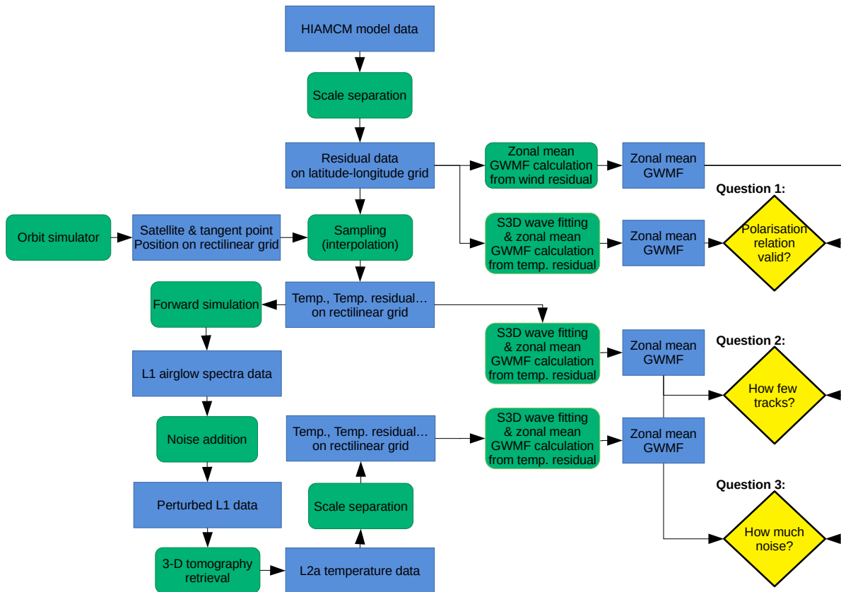
Figure 2. Schematic flow diagram of the assessment steps to address the three major questions highlighted in yellow diamond boxes. The assessment is based on comparison with zonal mean GWMF calculated directly from the model winds and considered here as the reference of truth. From top to down further assumptions and/or constraints are added as the tested data become more similar to the real observations.
