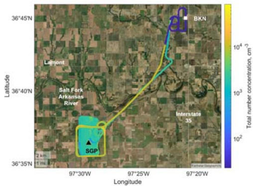
330 Figure 4. A typical flight track of one UAS flight (recorded on 2021/11/13) overlapped with the USGS national map. The UAS took off from Blackwell Municipal airport (BKN; white square) and sampled near the Central Facility (black triangle) of the SGP
