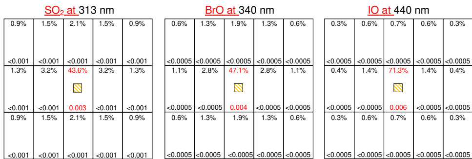
1180 Fig. 9 Horizontal coverage of a 1 x 1 x 1 km 3 plume (yellow hatched areas) by TROPOMI observations at different wavelengths. The numbers at the top of the TROPOMI pixels indicate the fractions of the plume molecules retrieved from that ground pixel. The numbers at the bottom indicate the optical depth of the trace gas absorption. Red values represent results above the respective detection limit.
