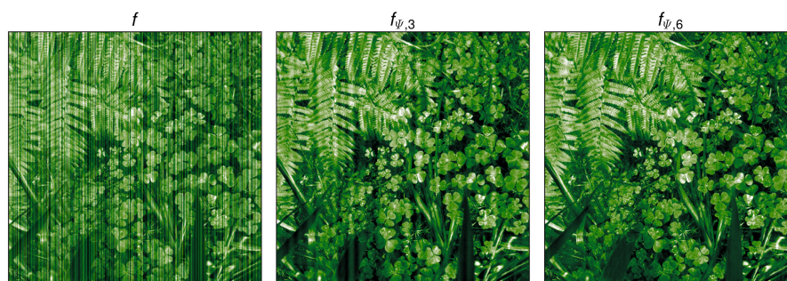
Figure 8. Performance of the combined wavelet-Fourier filter using Coiflet wavelets (coif16), \sigma = 2 , and different decomposition levels L .
