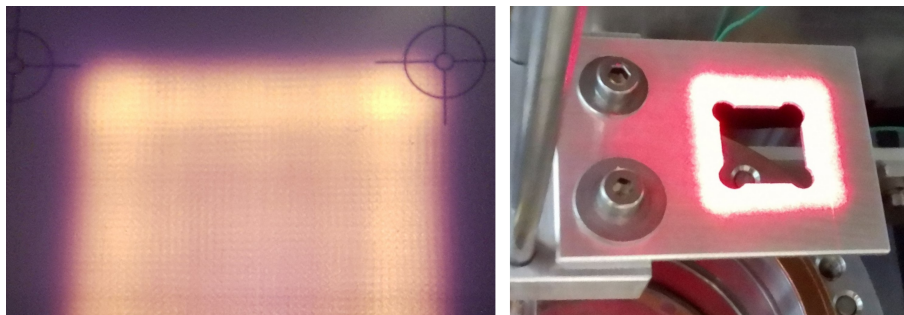
Figure 2. Left: Cross section of the laser beam (at 1530 nm) after passing through the homogenisation unit projected on a VRC4 IR detector card showing somewhat higher power densities at the edges. Right: Mask used to further shape the beam. The beam size of the visible trace laser is about 5 % larger than that of the NIR laser.
