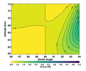
**648** Figure 5. Ozone twilight ratio, defined as  $O_3$  at solar zenith angle  $\theta/O_3$  at  $\theta=90^\circ$ , as a function of
