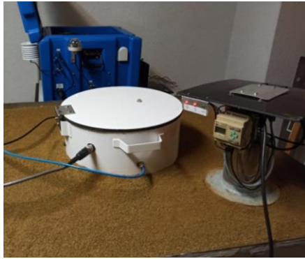
389 390 Figure 2. Typical calibration experiment carried out at the UC laboratory: the INTE_Flux system is installed together 391 with the TS system on the EB facility. 392
