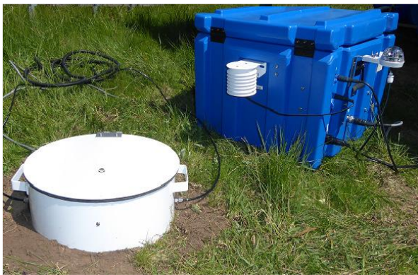
349 Figure 1. Image of the AutoFlux system running in the field. The radon activity concentration, internal air temperature, 350 differential pressure and soil characteristics are measured within the white drum. Ambient temperature, humidity, 351 pressure and rainfall are measured on the side of the transport case (~50 cm a.g.l.), and the main system components 352 are located inside the waterproof transport case.
