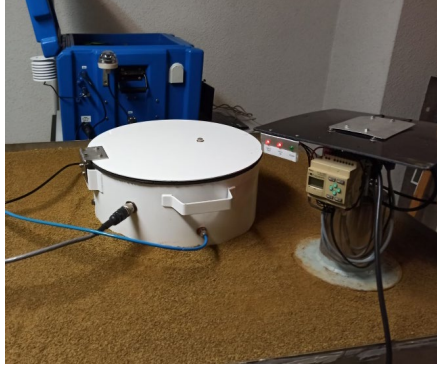
372 373 Figure 2. Typical calibration experiment carried out at the UC laboratory: the INTE_Flux system is installed together 374 with the TS system on the EB facility. 375
