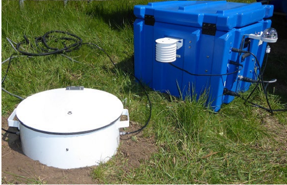
331 332 Figure 1. Image of the AutoFlux system running in the field. The radon activity concentration, internal air temperature, 333 differential pressure and soil characteristics are measured within the white drum. Ambient temperature, humidity, 334 pressure and rainfall are measured on the side of the transport case (~50 cm a.g.l.), and the main system components 335 are located inside the waterproof transport case.
