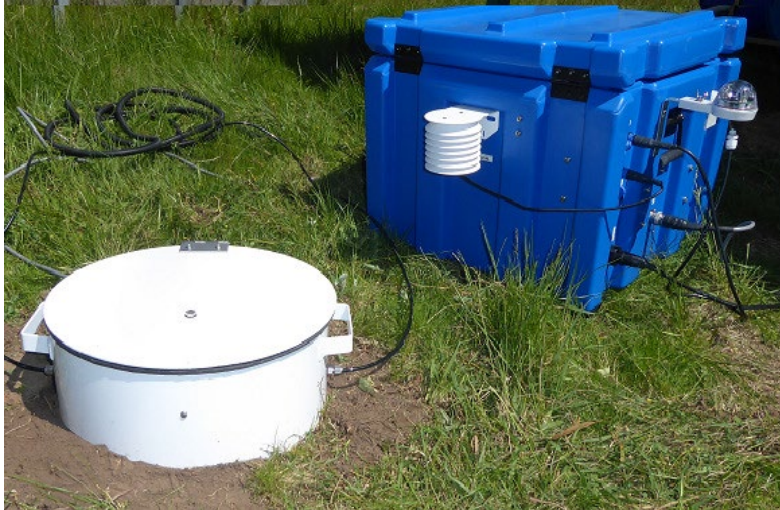
331 332 Figure 1. Image of the AutoFlux system running in the field. The radon activity concentration, internal air temperature, 333 differential pressure and soil characteristics are measured within the white drum. Ambient temperature, humidity, 334 pressure and rainfall are measured on the side of the transport case (~50 cm a.g.l.), and the main system components 335 are located inside the waterproof transport case.
