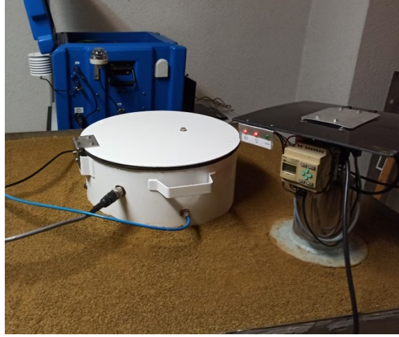
373 Figure 2. Typical calibration experiment carried out at the UC laboratory: the INTE_Flux system is installed together 374 with the TS system on the EB facility. 375
