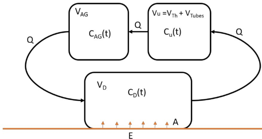
**Figure S8.** Conceptual box model of the ANSTO *AutoFlux* system.
