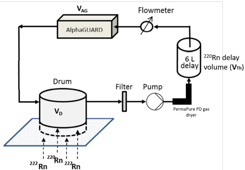
Figure S3. Schematic representation of the *AutoFlux* system (ANSTO).
