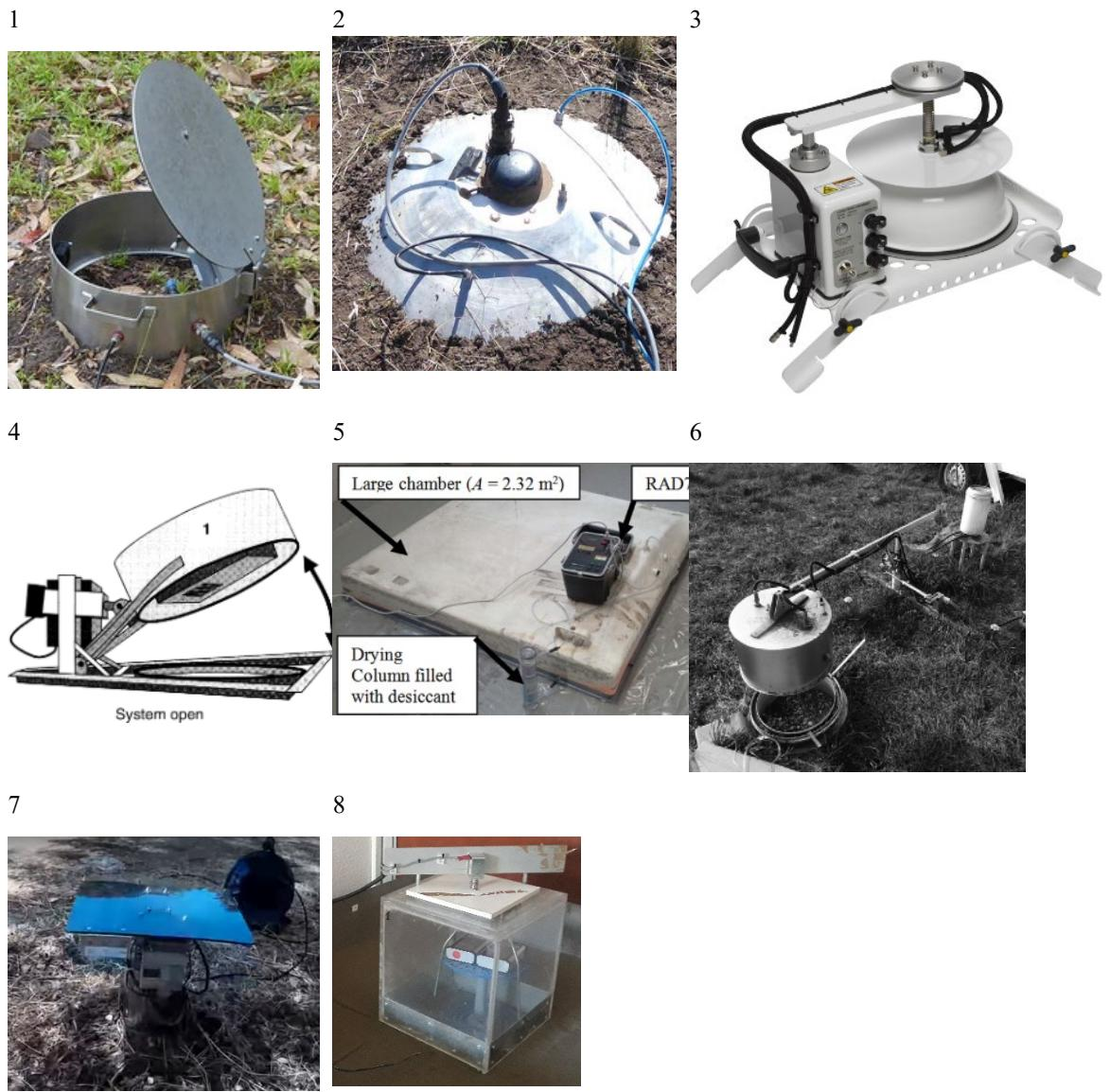
**Figure S2. Pictures of enlisted radon chambers, code numbers correspond to those in Table S4.**
