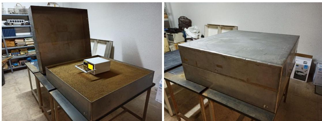
**Figure S1. Picture of the setup used to empirically determine the exhalation rate reference value of the EB.**
