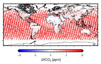
695 Fig. 10: Difference of XCO<sub>2</sub> between V03.00 and the bias-corrected one (bias-corrected minus V03.00) averaged from the launch to 2021 within a 2.5°×2.5° grid.
