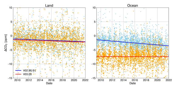
690 Fig. 9: Time series of the differences between GOSAT and in situ measurements (GOSAT minus in situ measurements) over land (left) and the ocean (right). The differences in monthly averaged values for V02.90/91 (light blue) and V03.00 (orange) in each area are plotted. The regression lines are plotted as the blue and red lines.
