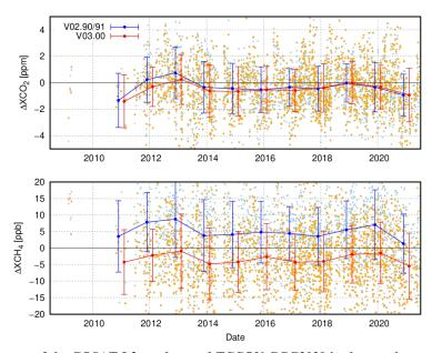
Fig. 7: Annual mean differences of the GOSAT L2 product and TCCON GGG2020 in the match-up condition of ±0.1°. for XCO2 (top) and XCH4 (bottom). The red and blue lines indicate V03.00 and V02.90/91, respectively. The annual mean plots are slightly shifted between V02 and V03 for visibility. Each individual observation from V03.00 and V02.90/91 is plotted as orange and light-blue dots.
