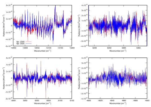
Fig. 1: Averaged spectral residuals (simulated minus observed) at O<sub>2</sub>A (top-left), WCO<sub>2</sub> (top-right), CH<sub>4</sub> (bottom-left), and SCO<sub>2</sub> (bottom-right) sub-bands in April 2009 (red) and April 2020 (blue) over land obtained from V02.90.
