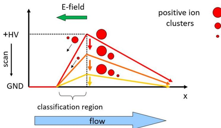
415 Figure 1. Principle of the axial ion mobility classifier (AMC). An electric field is opposed to the flow direction. The strength of the electric field decreases from red to yellow. Scanning of the voltage allows to determine the half-pass mobility of a specific ion. The half-pass mobility is found at the voltage where one half of the number concentration of this ion is able to pass the potential barrier.
