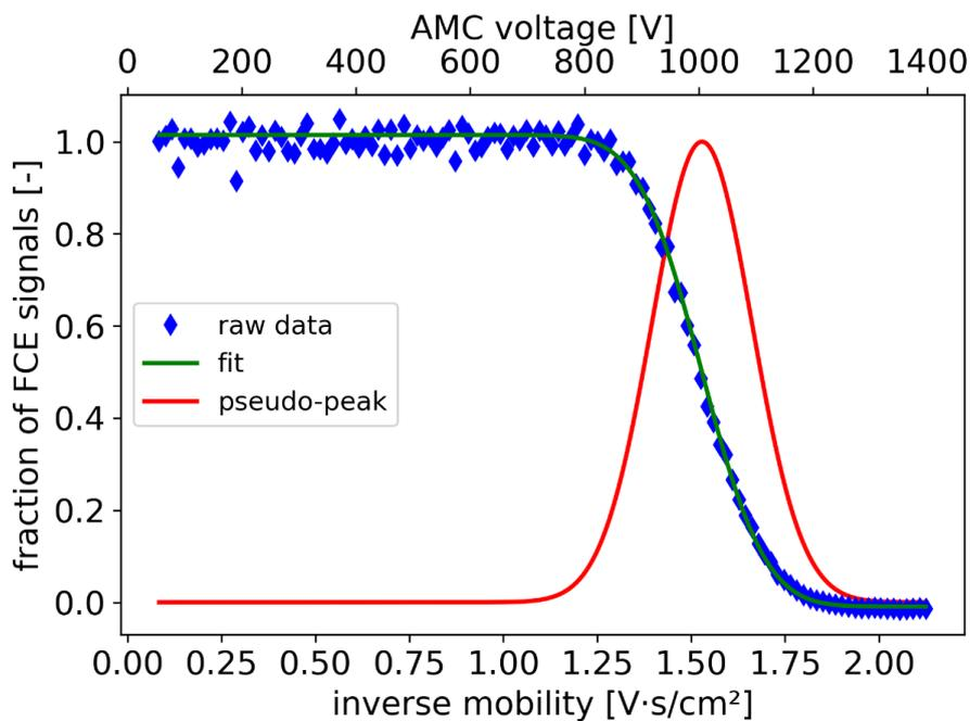
440 Figure 5. Example AMC scan of THAB dimer showing the relative transmission efficiency i.e., the fraction of FCE signal after the AMC (FCE2) divided by the FCE in front of the AMC (FCE1), as a function of the scanning voltage. Raw data presented in blue follows a sigmoidal relationship displayed as green line. The derivative of the fitted sigmoidal function multiplied by -1 yields a pseudo-peak shown in red.
