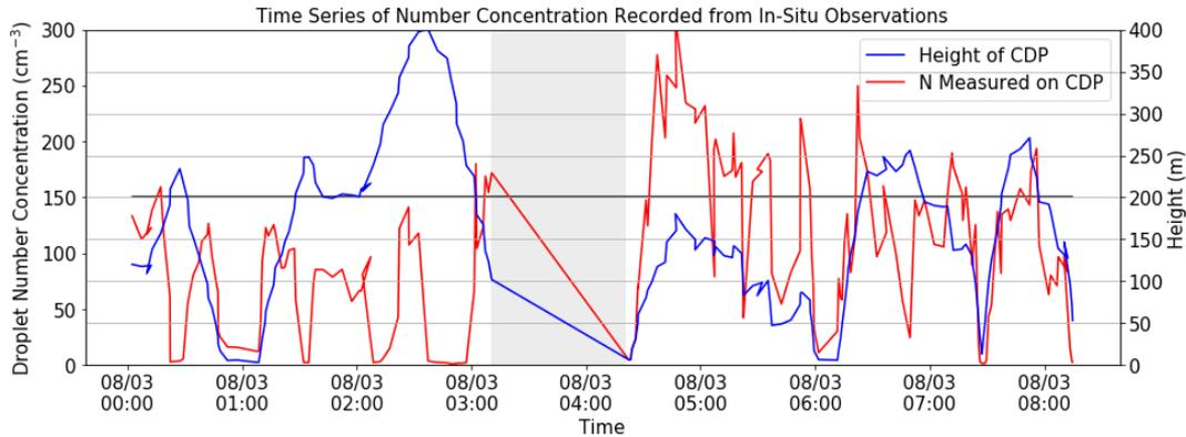
**Figure 8.** The total cloud droplet number concentration recorded by the CDP throughout the fog event observed on the 7 - 8 March 2020, with the height of the instrument shown on the same graph. The number concentration assumed in the retrieval of  $150 \text{ cm}^{-3}$  is highlighted with the black line.
