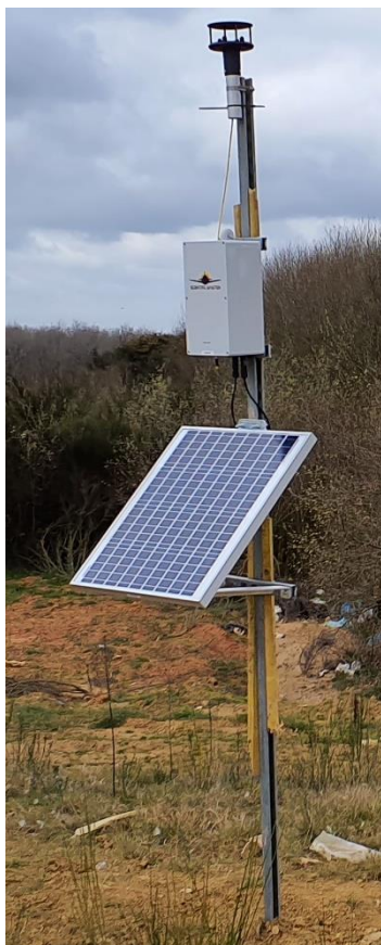
Figure 3: System A autonomous field logger (LSCE007) installed at the SUEZ Amailloux landfill site in March 2021 (see text for description). This system includes a two-dimensional anemometer.
