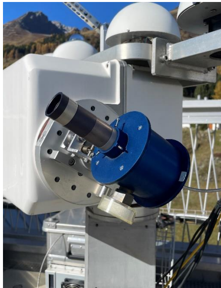
670 Picture 1: The lens-based telescope of Koherent on a sun tracker at the measurement platform of PMOD/WRC. The telescope is connected by an optical fiber to the BTS array spectroradiometer in the temperature stabilized box.
