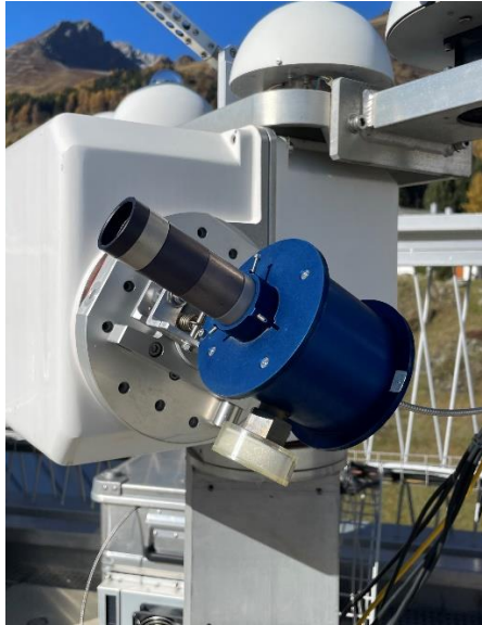
675 Picture-Figure 1: The lens-based telescope of Koherent on a sun tracker at the measurement platform of PMOD/WRC. The telescope is connected by an optical fiber to the BTS array spectroradiometer in the temperature stabilized box.
