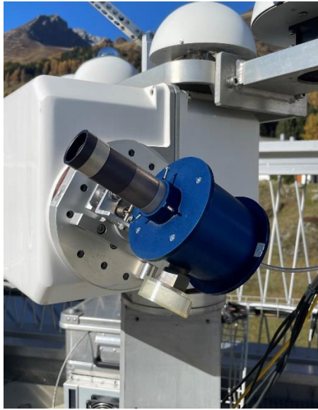
Figure 1: The lens-based telescope of Koherent on a sun tracker at the measurement platform of PMOD/WRC. The telescope is connected by an optical fiber to the BTS array spectroradiometer in the temperature stabilized box.
