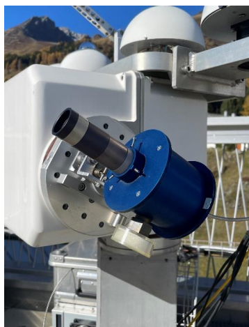
Picture 1: The lens-based telescope of Koherent on a sun tracker at the measurement platform of PMOD/WRC. The telescope is connected by an optical fiber to the BTS array spectroradiometer in the temperature stabilized box.
