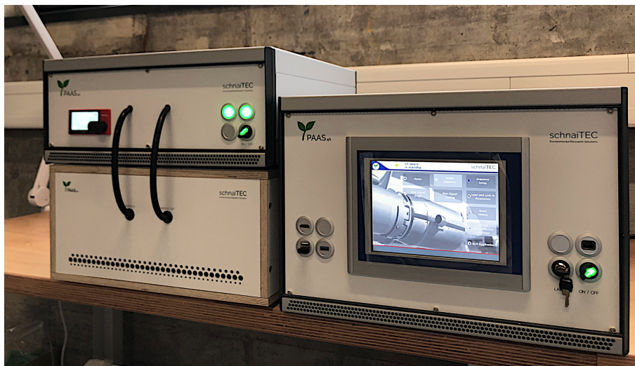
Figure S1. Photograph of the PAAS-4 \lambda consisting of the Optics Unit (lower left ), the Flow Unit (upper left), and the Electronics Unit (right).
