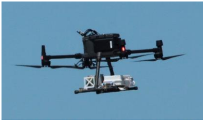
Figure 1. Picture of the AUSEA 112 analyzer mounted on a DJI M300.
