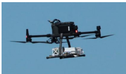
915 Figure 1. Picture of the AUSEA 112 analyzer mounted on a DJI M300.
