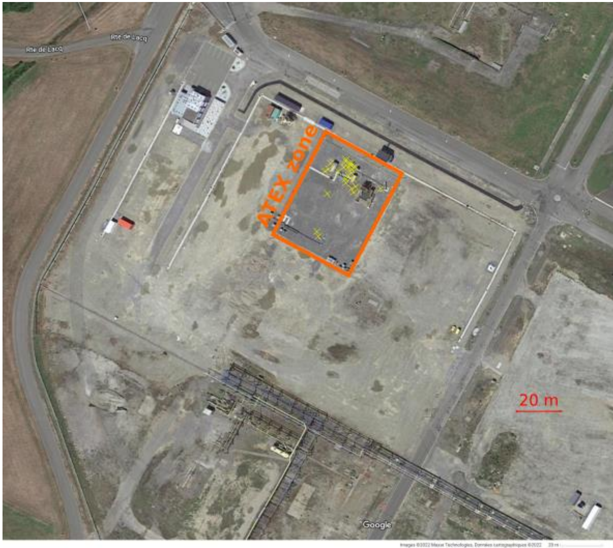
Figure 5. Aerial view of the TADI platform with location of the emission sources (yellow crosses) and the Explosive Atmosphere area (ATEX zone, depicted as an orange square). Maps Data: Google, ©2022 Maxar Technologies.
