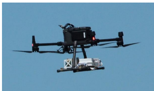
Figure 1. Picture of the AUSEA 112 analyzer mounted on a DJI M300.
